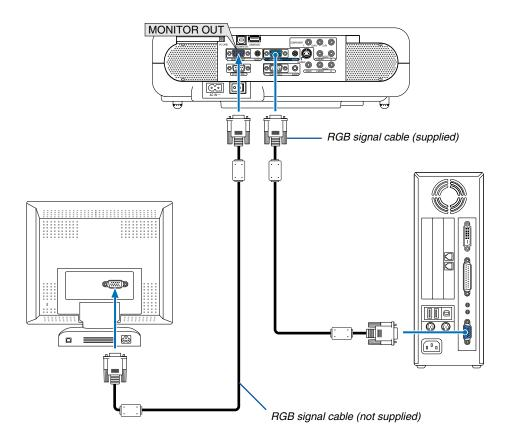
You can connect a separate, external monitor to your projector to simultaneously view on a monitor the RGB analog image you're projecting.
